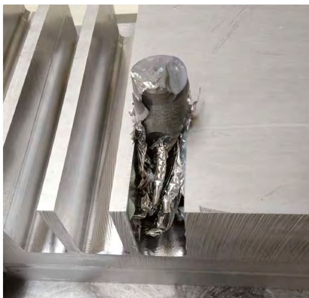
Safe-Lock で工具の抜け防止 No pull out of the tool with Safe-Lock
