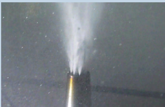
Cool Flash—効果的に刃先冷却 Cool Flash – effective cooling at the cutting edges
